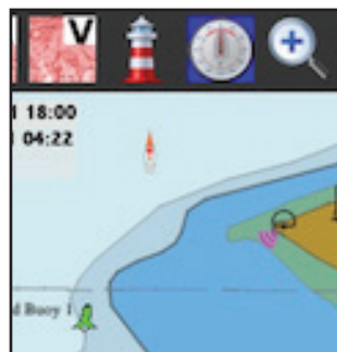
Figure 3-2. Lighthouse icon in the toolbar. This only shows up in vector chart mode, but it is a handy tool when shown.
