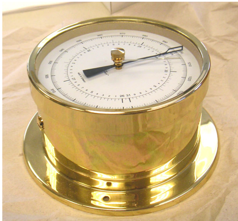
Fischer Precision Aneroid Barometer provides pressures to \pm 0.7 mb without an extra calibration curve.
