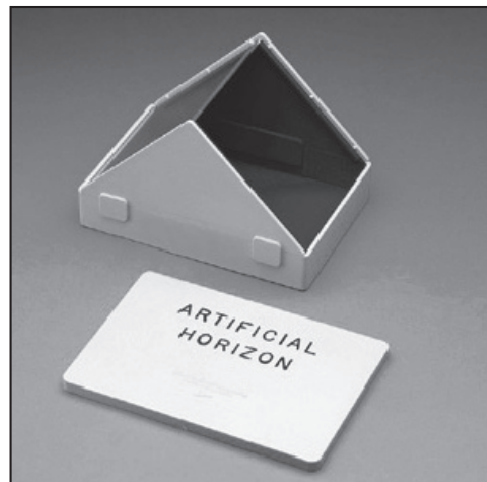
Figure 11.19-1 Davis artificial horizon, about 4 inches wide, about $30.
